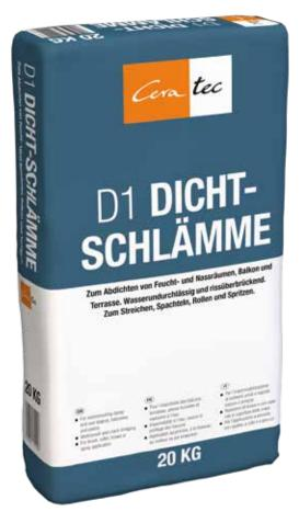
Mineral, flexible slurry seal for waterproofing showers, toilet facilities in accordance with DIN 18534 and for the sealing of containers and tanks in accordance with DIN 18535 Part 3.
